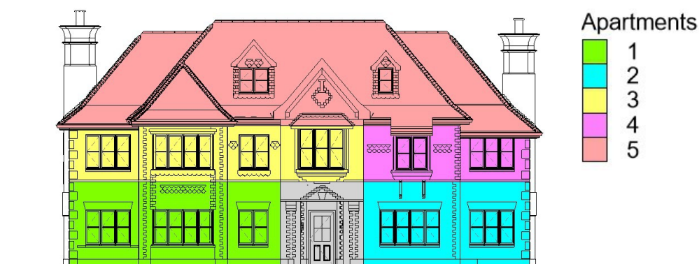
Drawing 3.1.7b above shows the newly revised scheme with only 5 apartments (with the previous basement apartments removed from the scheme.)
