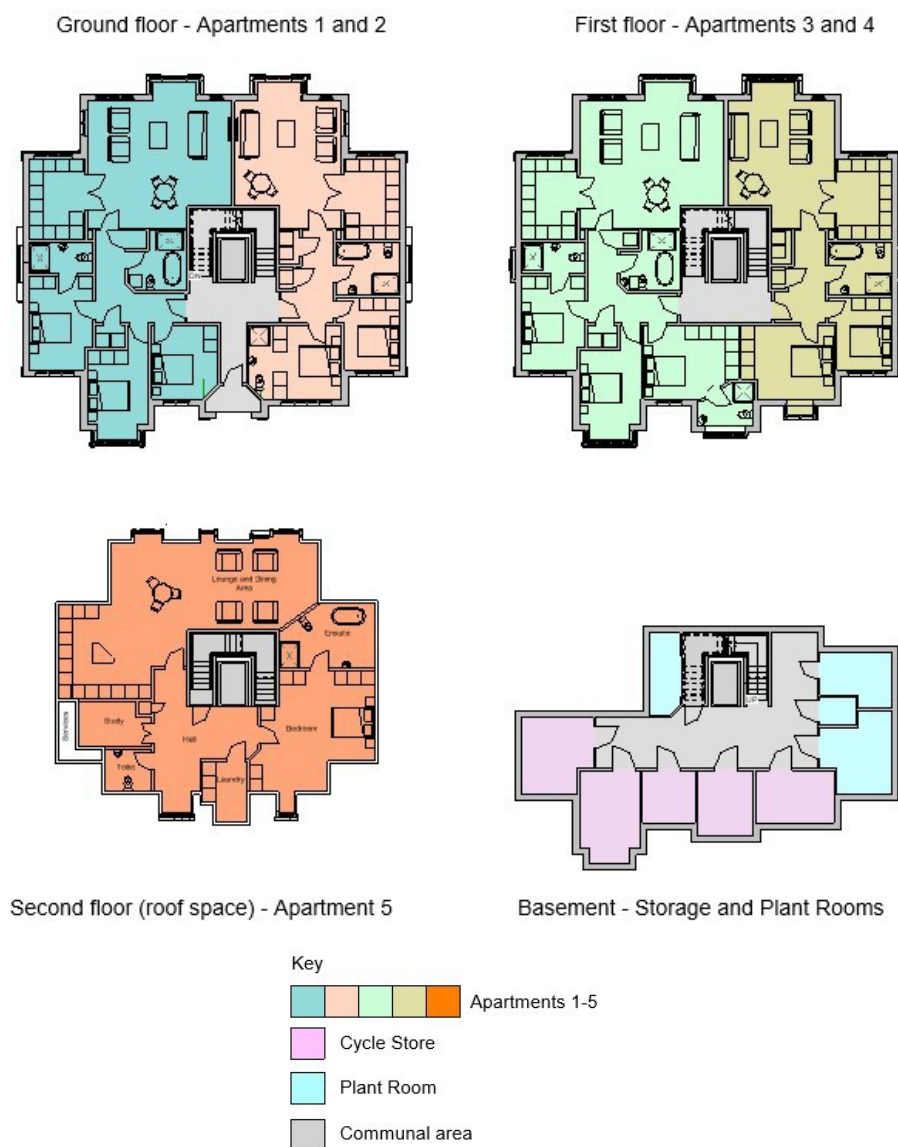
Drawing 4.6a above shows the revised proposed floor plans.
