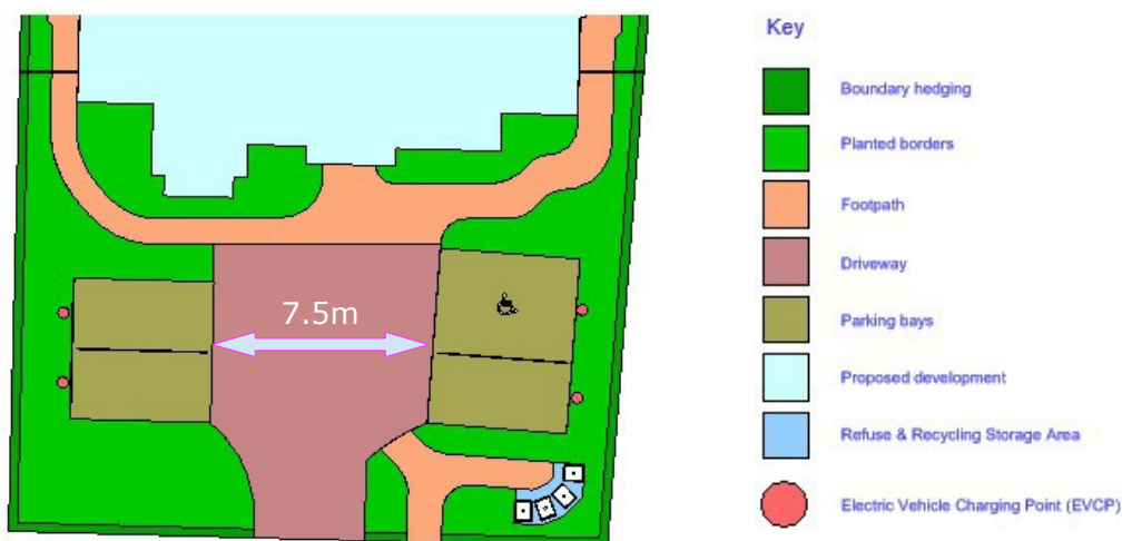
Drawing 4.7b above shows the newly proposed site plan with an equal access parking bay designed into the scheme.
