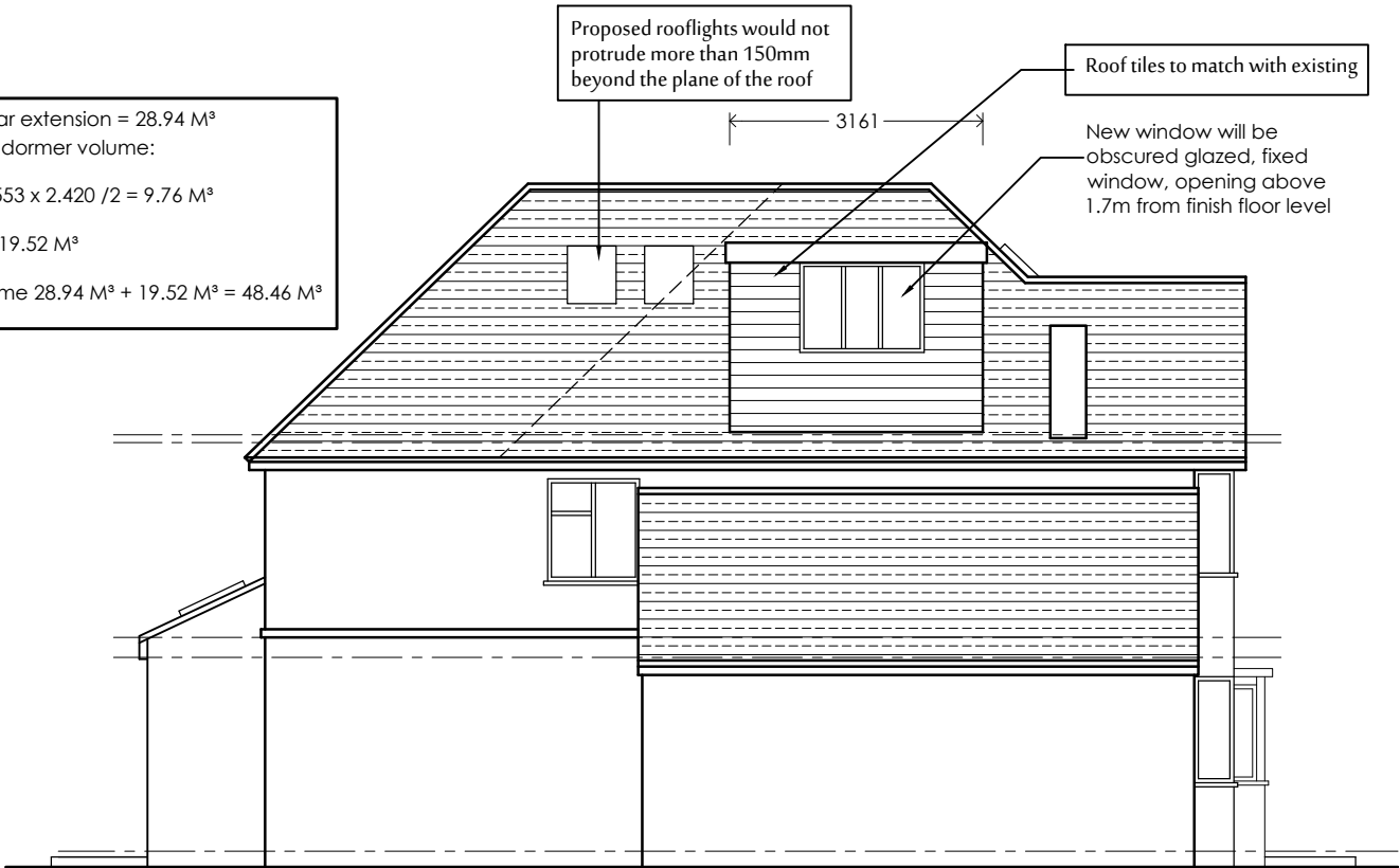
SIDE ELEVATION FACING No 57
