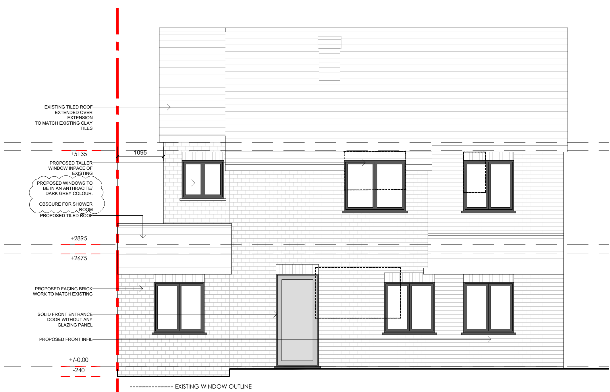
PROPOSED Front Elevation scale 1:50 @ A1
