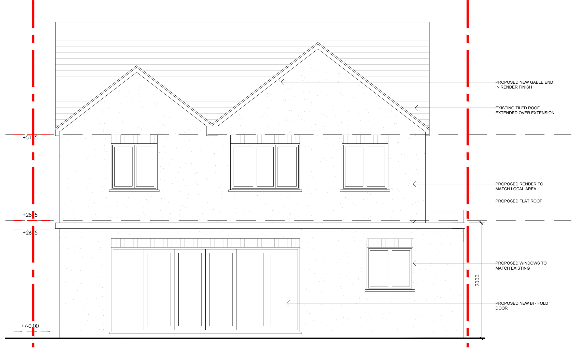
PROPOSED Rear Elevation scale 1:50 @ A1
