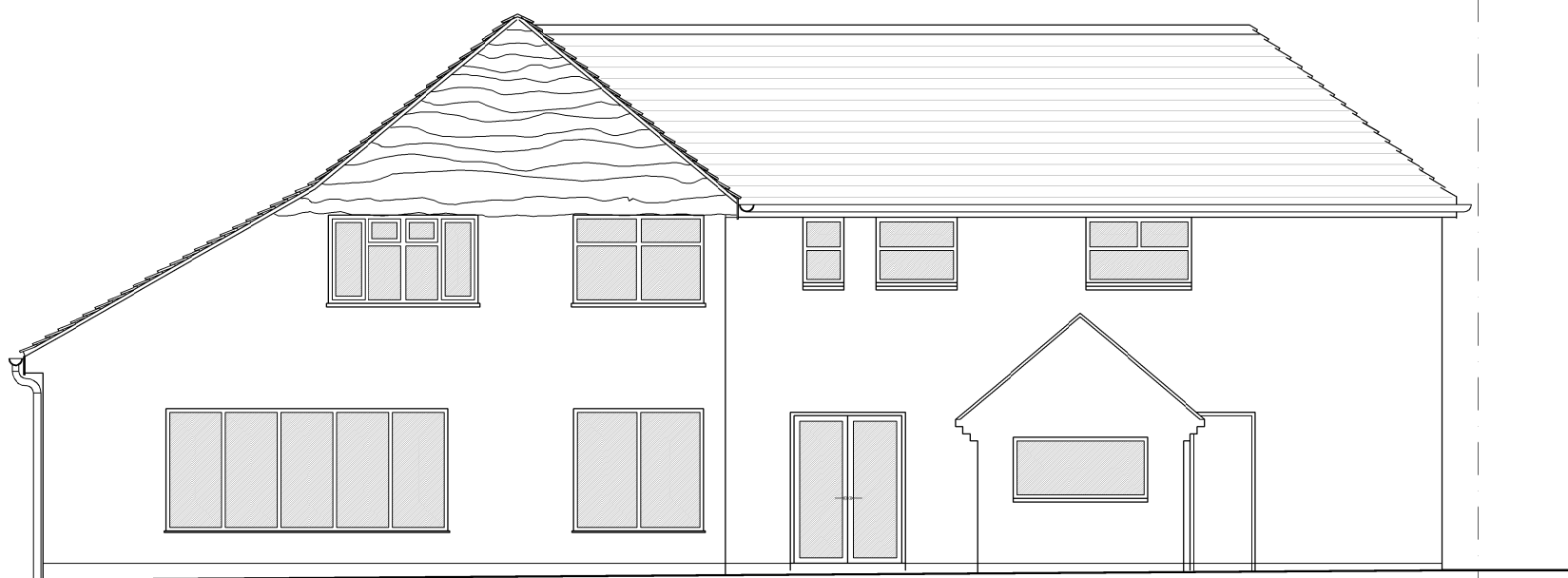
EXISTING: REAR ELEVATION
