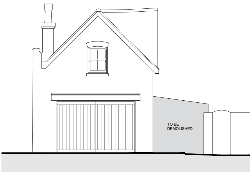
EXISTING FRONT ELEVATION
