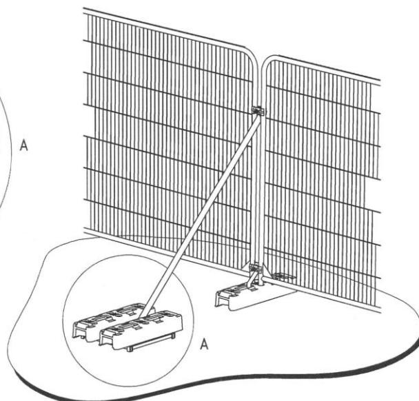
b) Stabilizer strut mounted on block tray
