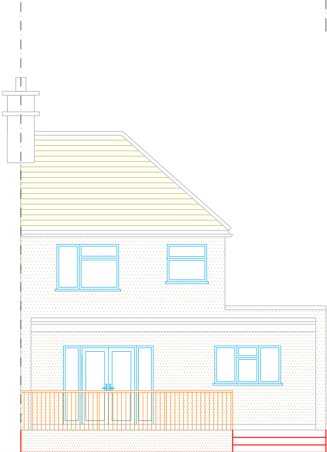
EXISTING REAR ELEVATION
