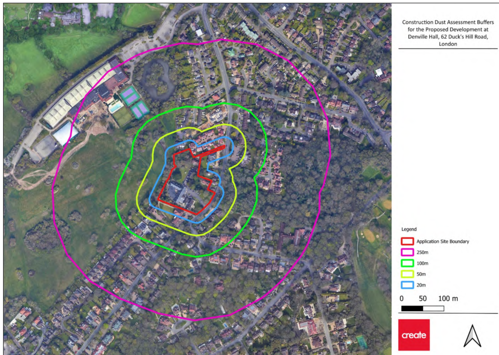
Figure 4.1: Construction Dust Assessment Buffer Zones
