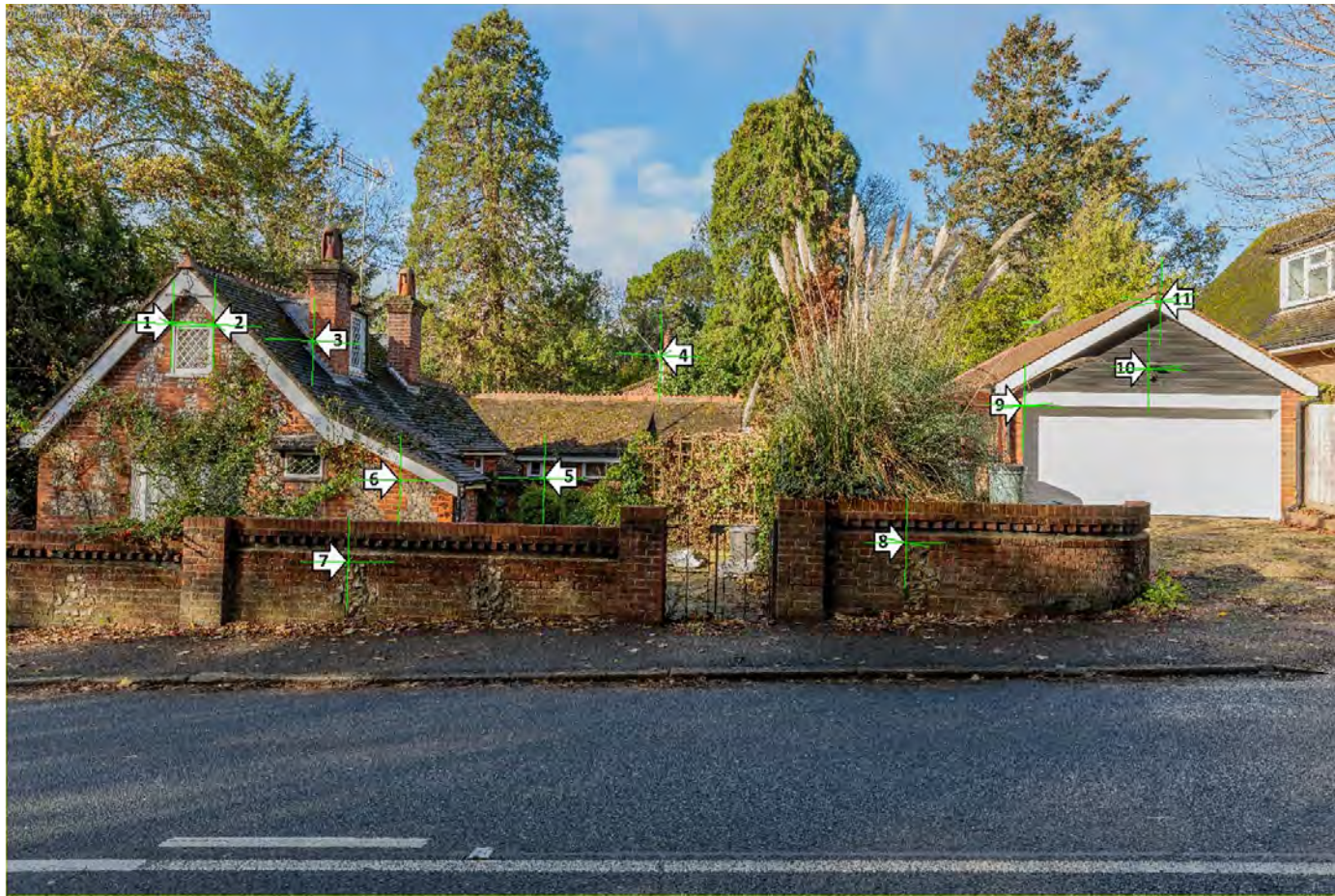
VERIFIED CAMERA VIEW Annotated key points (white arrows) and their corresponding survey points (green crosses) seen through the re-created virtual camera demonstrating a verified view.
