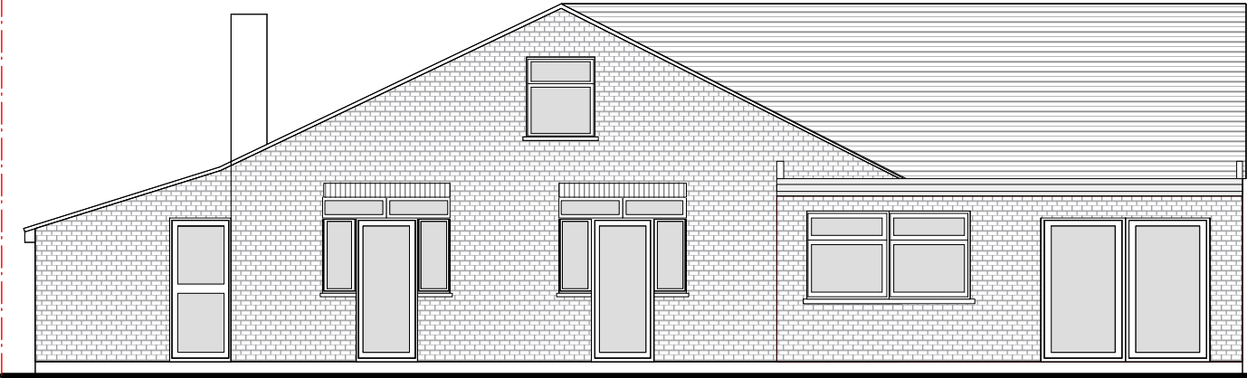
1 EX-20 REAR ELEVATION Scale: 1/100
