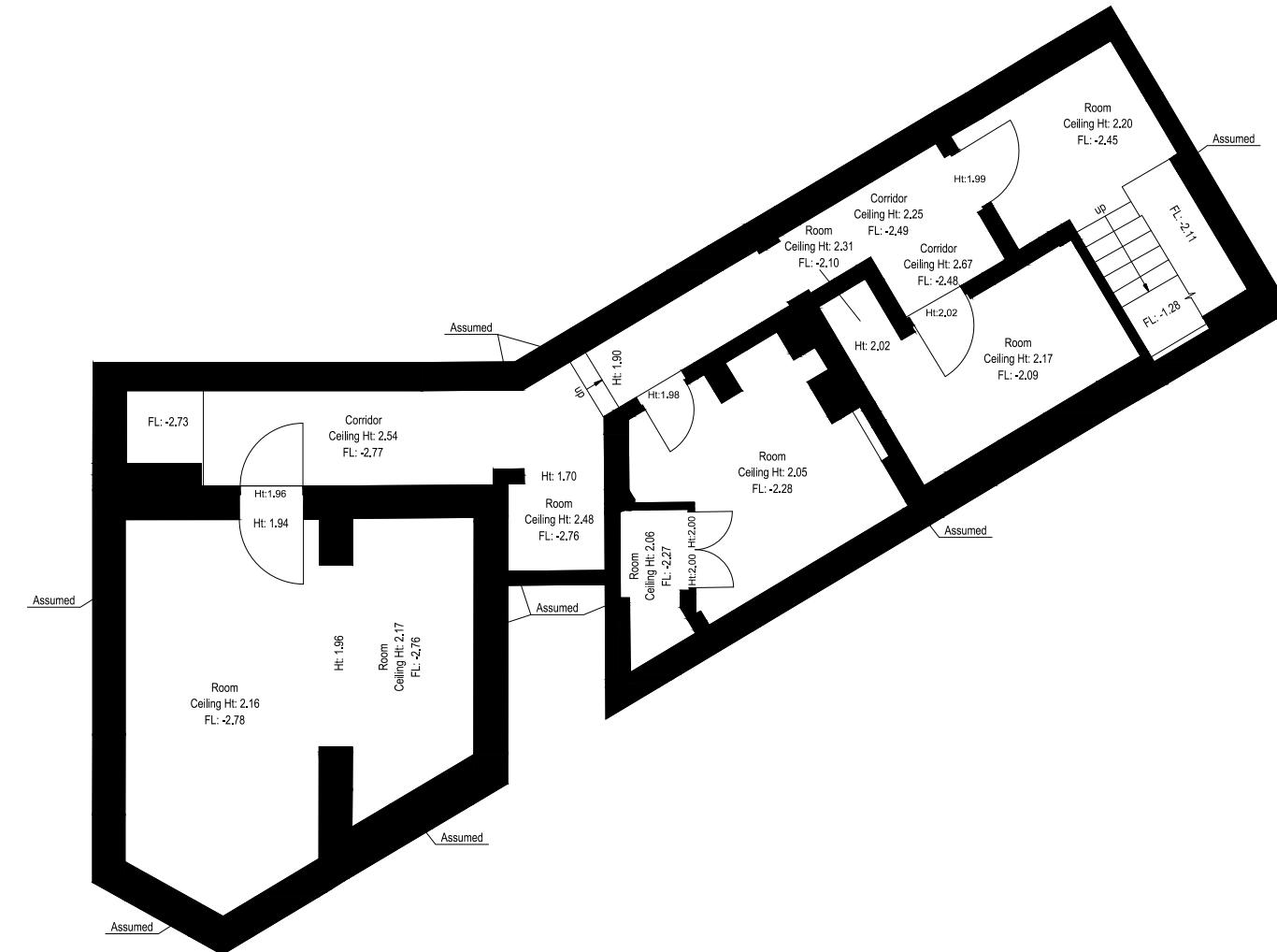
Proposed Basement Floor Plan (as existing)
