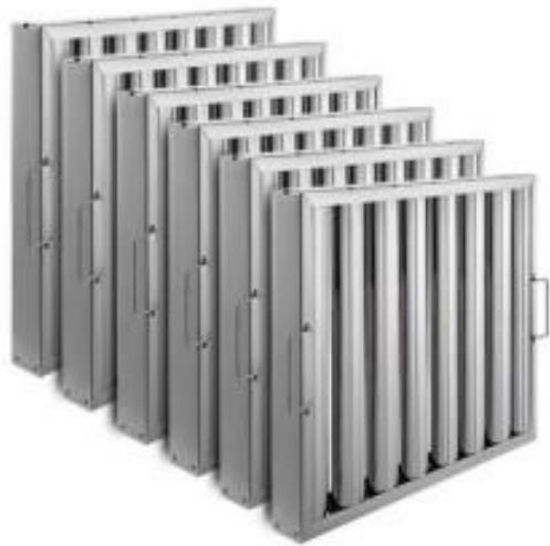
These Grease baffle filters are made from stainless steel for easy cleaning and are extremely effective at removing airborne grease particles before they enter the ductwork. With their unique design and interlocking baffles, they change the direction of grease laden air which also restricts flames from entering into the ductwork.
