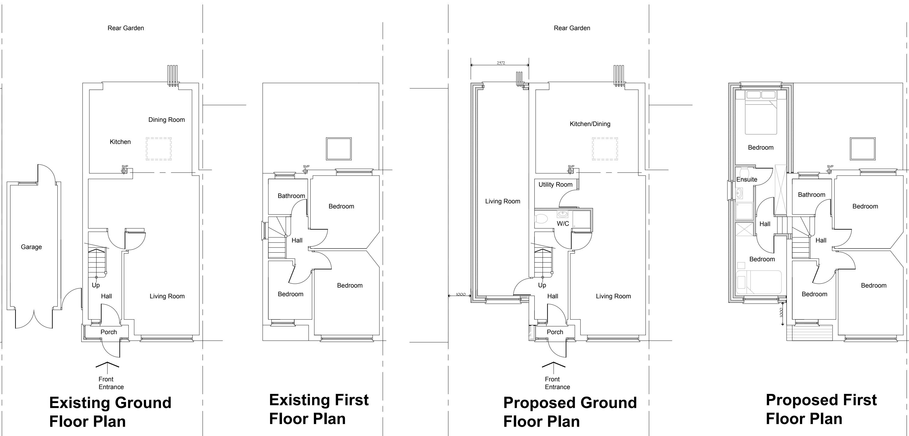
This is a 'Scheme Level Drawing' and is intended to illustrate the general arrangement of the project proposals. As it stands this drawing does not include all of the detail necessary for a full plans building regulations application.
