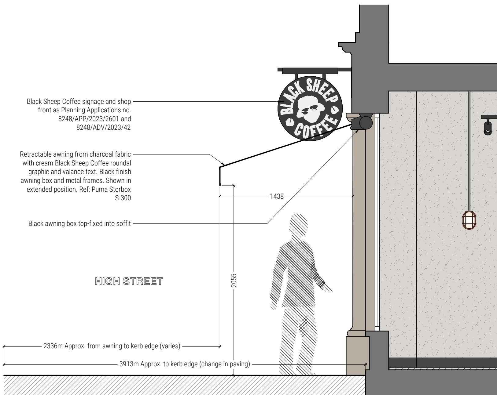
Section A: Typical Section Through Shop Front
