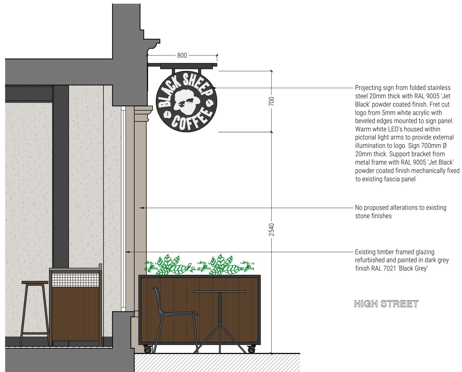
Section A: Typical Section Through Shop Front
