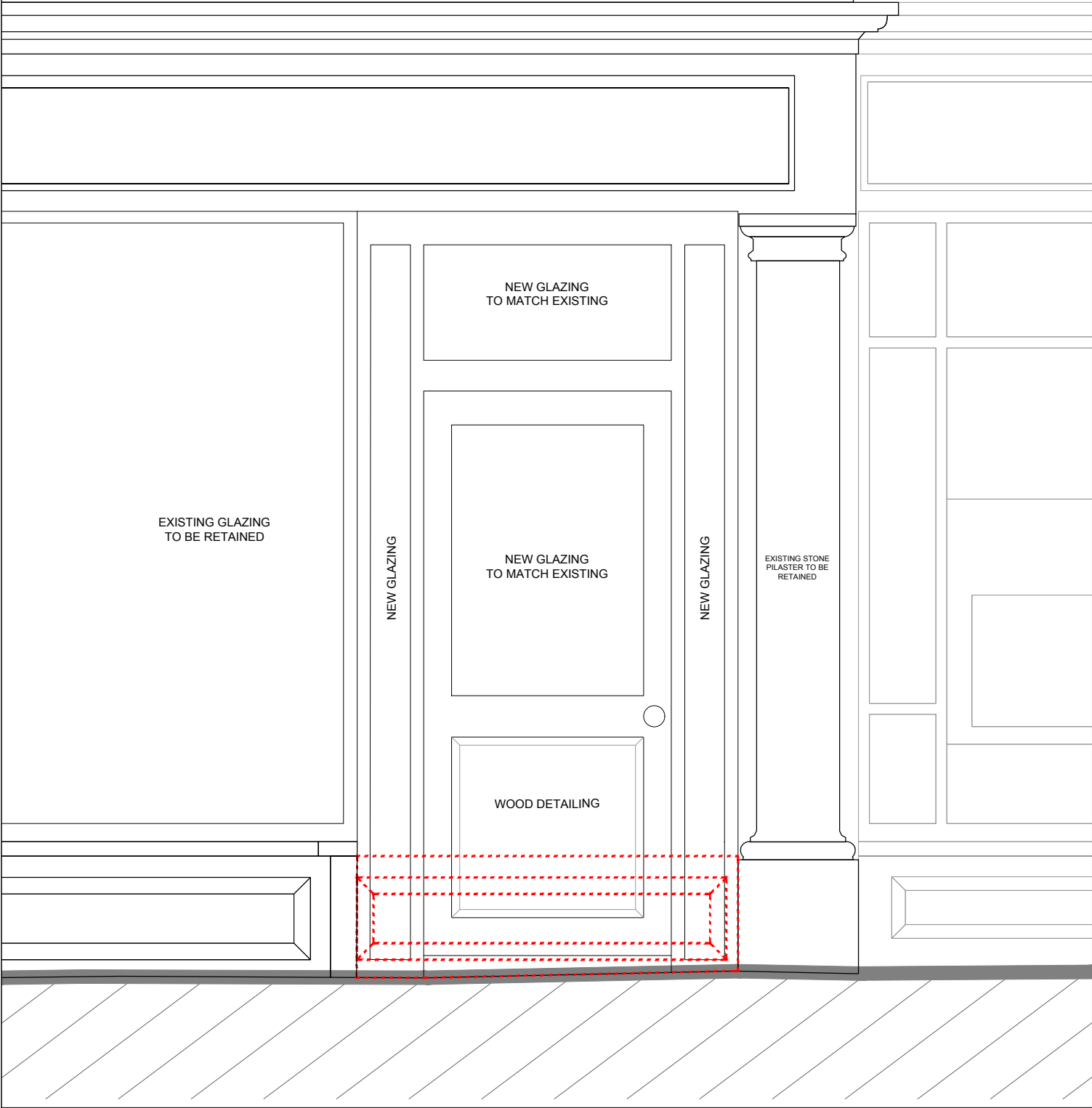
The image above (taken 22/03/2023) shows the area of the existing glazing and stone plinth that will be carefully removed to make way for the new entrance way.
