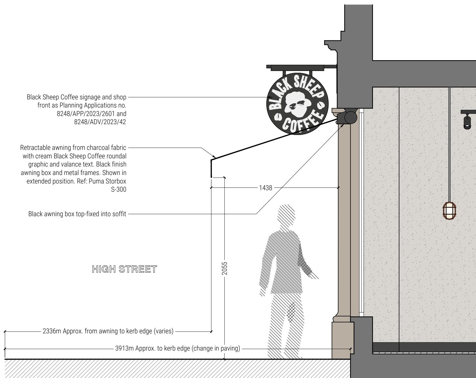
Section A: Typical Section Through Shop Front
