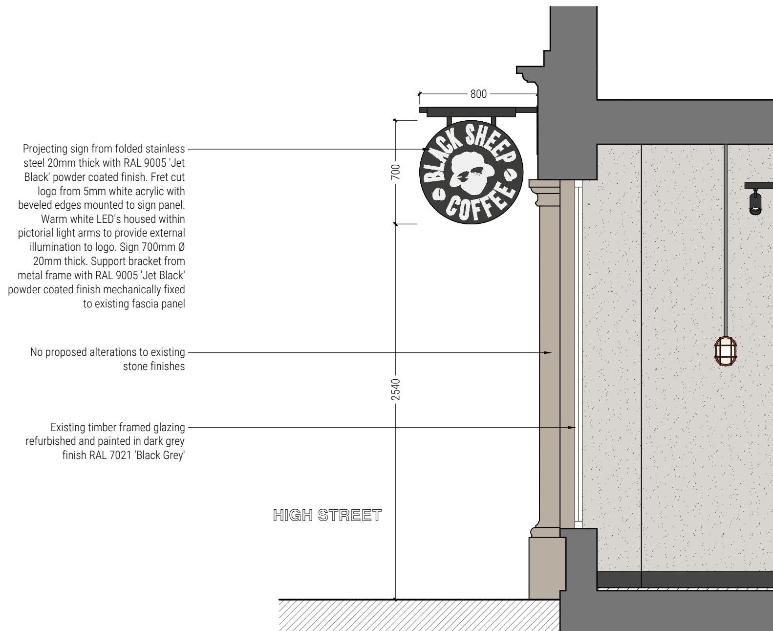
Section A: Typical Section Through Shop Front
