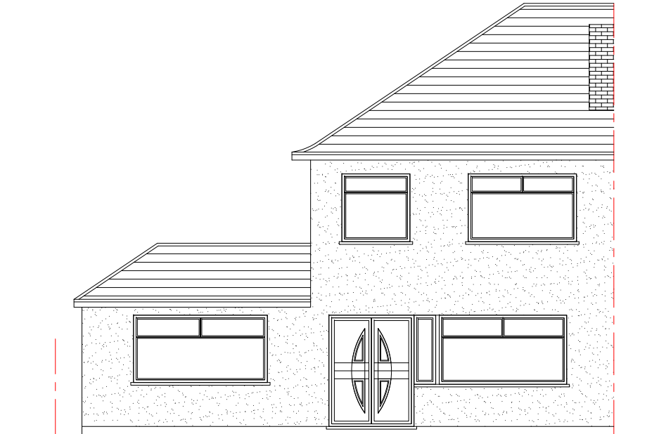
Existing Front Elevation Scale 1:100
