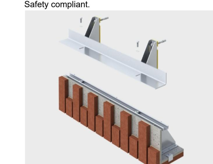
B.O.S.S. A1 is a lightweight, carbon neutral, pre-fabricated brick slip soffit system designed to be quickly and easily bolted to IG's Welded Masonry Support (WMS) to create spectacular brick soffits. This BBA certified unit is manufactured completely from A1 fire rated materials and is Document B:Fire Safety compliant.
