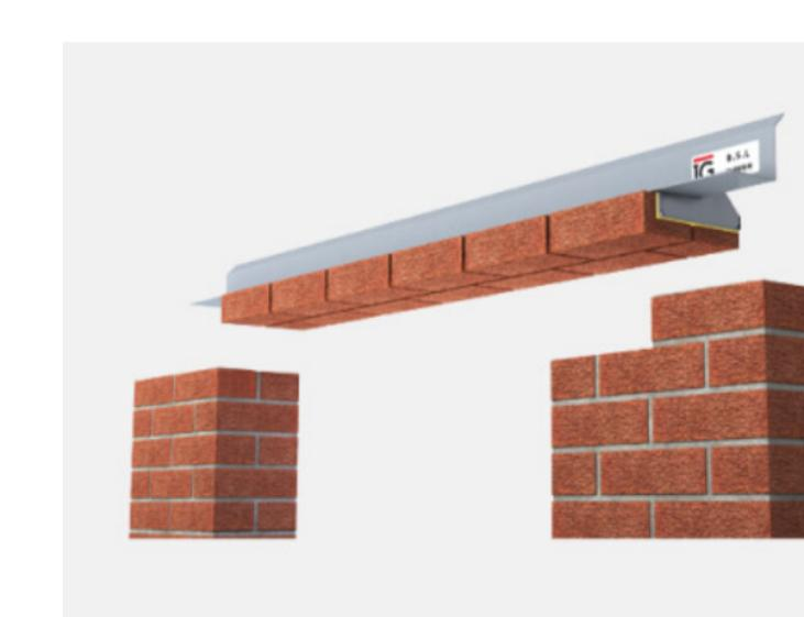
IG Brick Slip Lintels are a lightweight, stainless steel, pre-fabricated brick slip unit designed for openings up to 3.6 metres. Manufactured off-site, the units are delivered to site complete with brick slips bonded to the stainless steel carrier unit.
