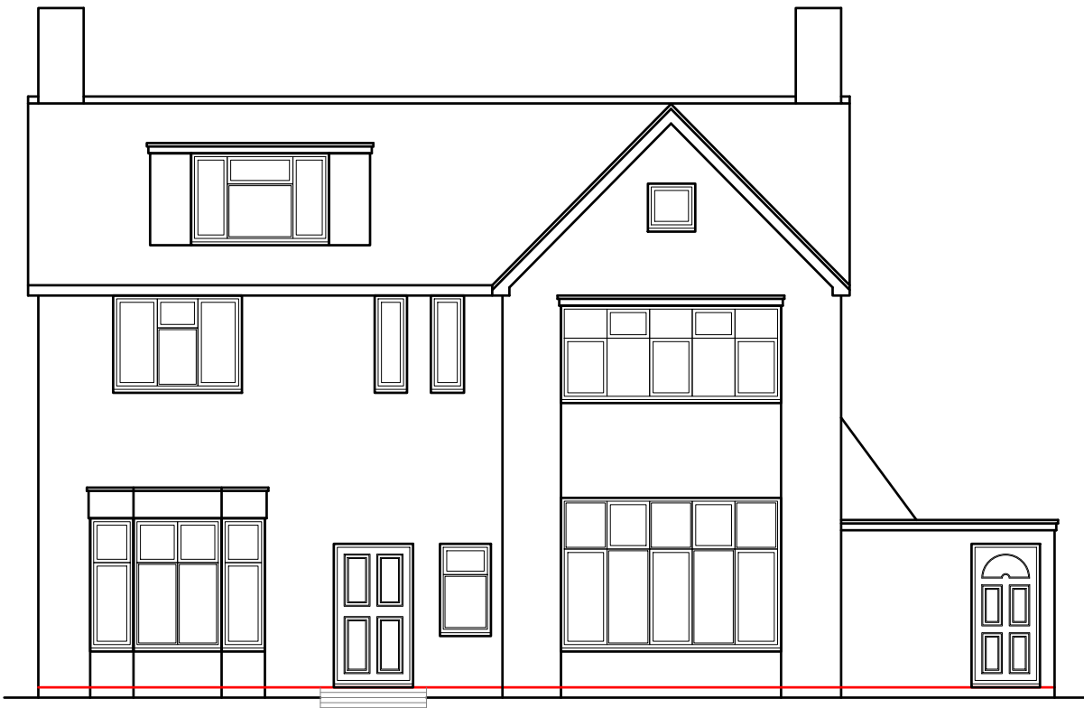
PRE-EXISTING FRONT ELEVATION 1:100
