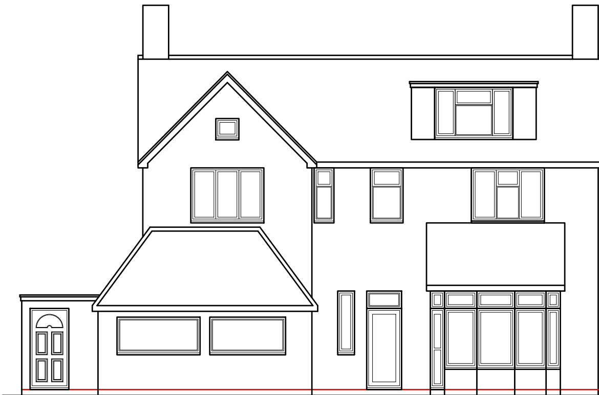
PRE-EXISTING REAR ELEVATION 1:100
