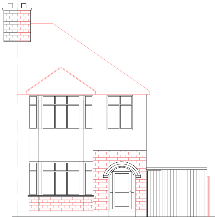
FRONT ELEVATION (existing)
