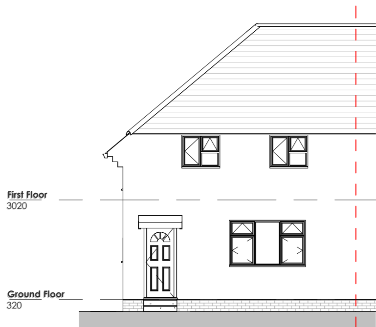
Existing Front (NW) Elevation @ 1 : 100
