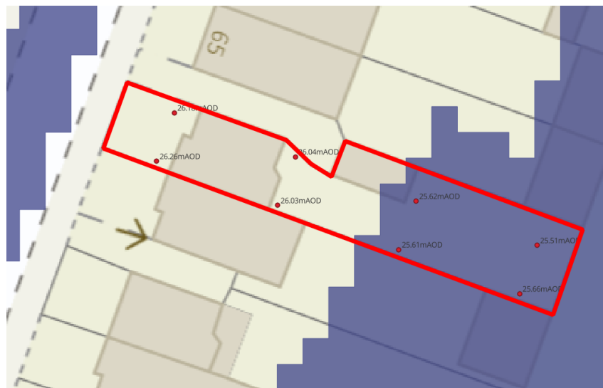
Figure 8: Spot levels on site relative to the areas of 1 in 100yr + CC flood risk. The transition occurs at c25.8m AOD
