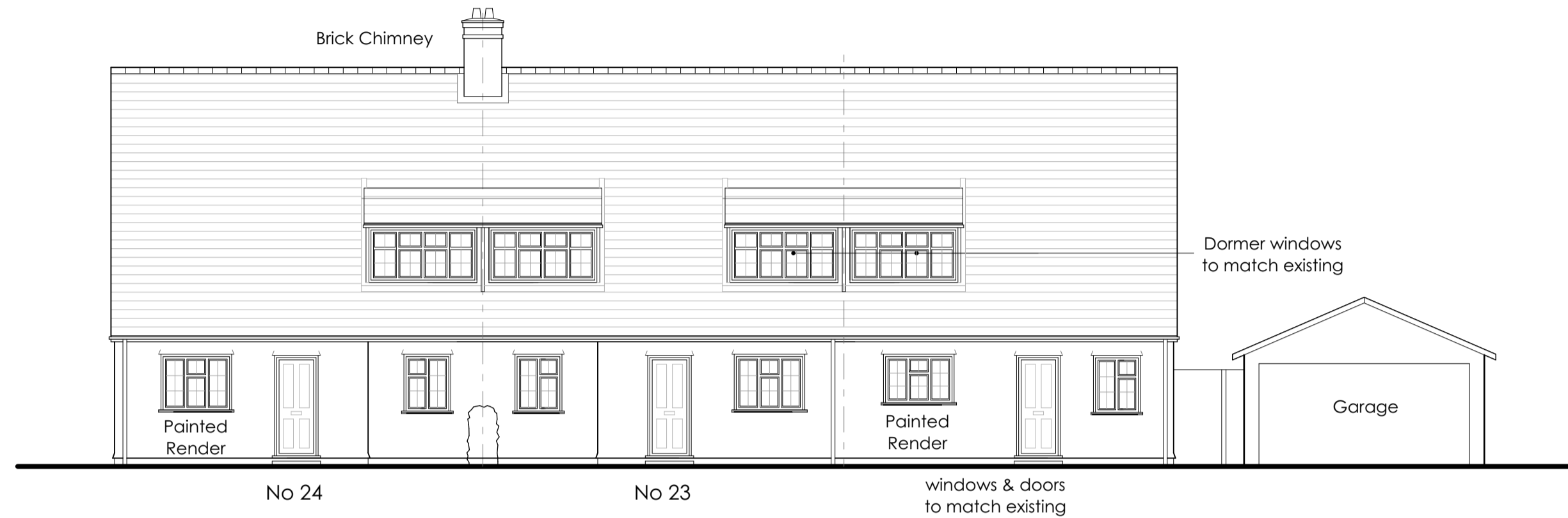
Front Elevation - South Facing Green Walk
