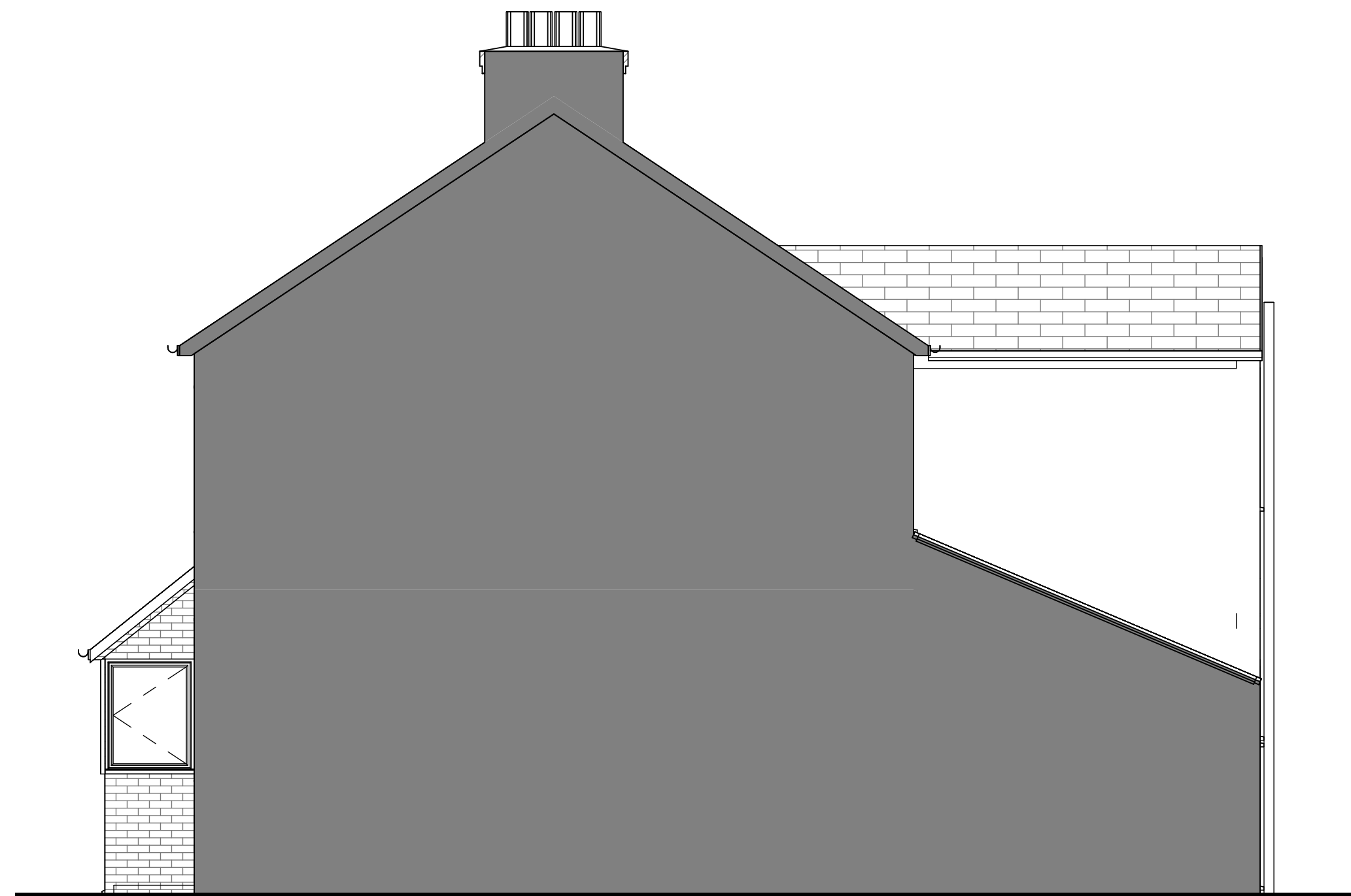
EXISTING SIDE ELEVATION 1 : 50
