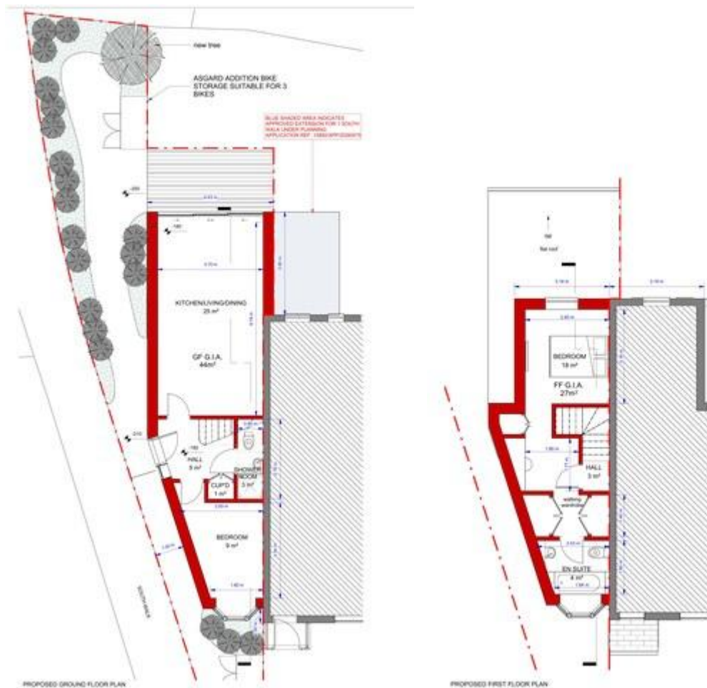
Proposed ground and first floor plans, drawing 25102-03 Rev B. The blue shaded area indicates the approved rear extension at No. 1 South Walk (ref. 14892/APP/2026/675), with which the rear building line aligns
