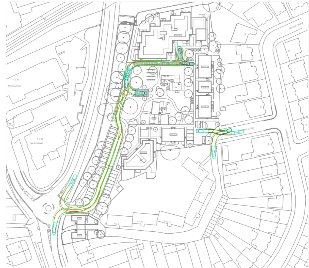
Figure 6 – Indicative Fire Service Vehicle Access
