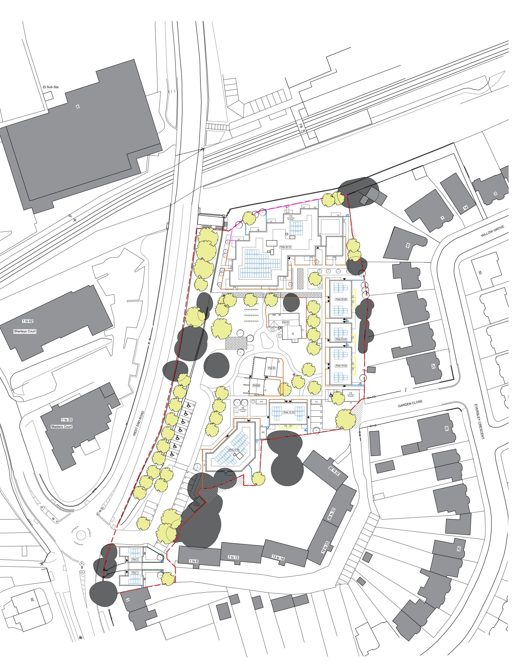
**KEY Application Boundary** Adjacent Land in Client Ownership Trees Existing Trees New 1.8m High Closed Boarded Timber Fence 0.9m High Metal Estate Railings with Hedge behind 1.8m High Metal Railings 0.45m Knee Rail 2.1m High Brick Wall RCP Refuse Collection Point CS Cycle Store Hardstanding Emergency Access Only Indicative PV Indicative PV Location
