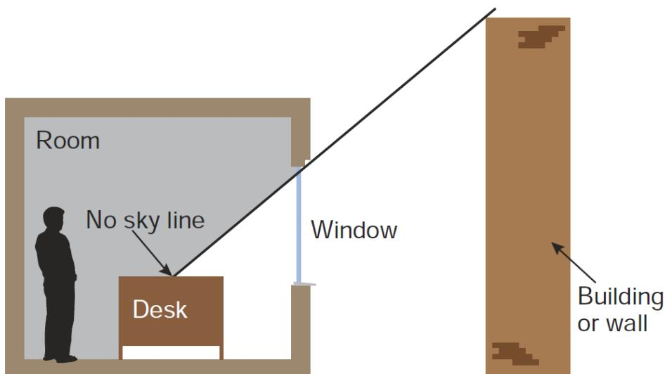
**Figure 4 - The no-sky line divides areas of the working plan which can and cannot receive direct skylight.**
