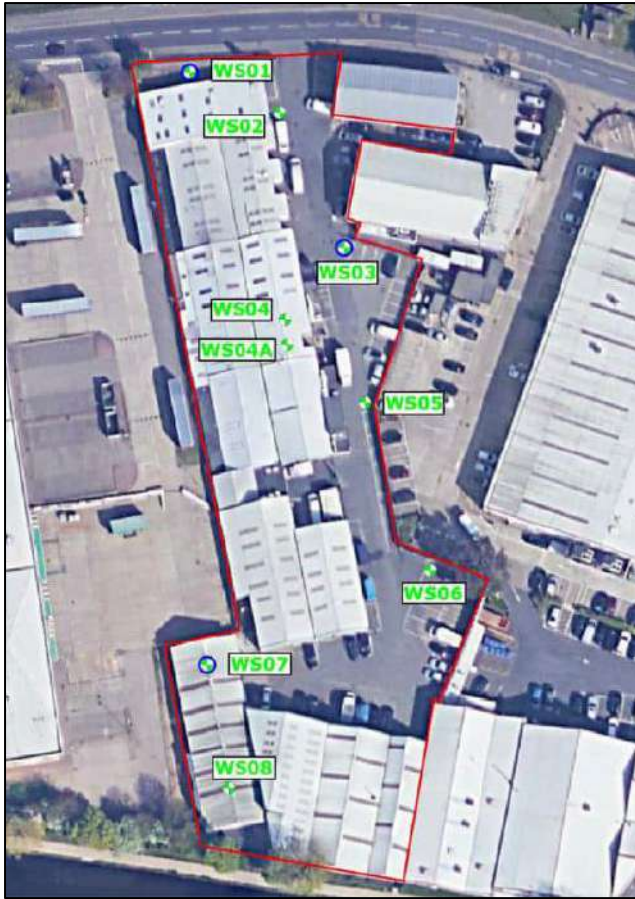
Figure 5 - Windowless Borehole Location Plan (Ground Condition Assessment, Ridge 2025)
