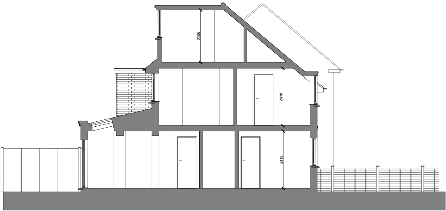
SECTION BEECH AVE 11 AS PROPOSED SCALE 1:50
