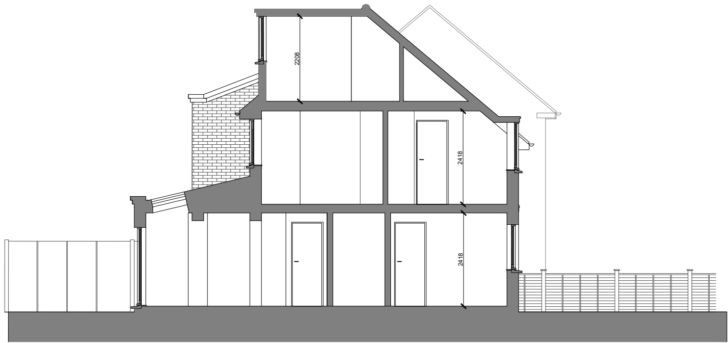
SECTION BEECH AVE 11 AS PROPOSED SCALE 1:50
