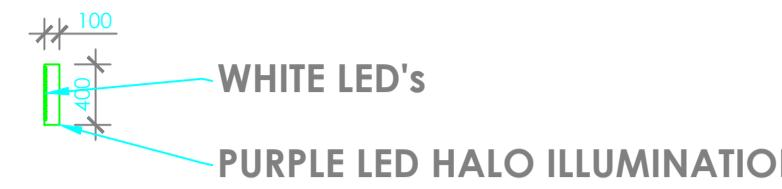
**proposed** Taco Bell Letters mounted on raceway (Sign No.1) -
