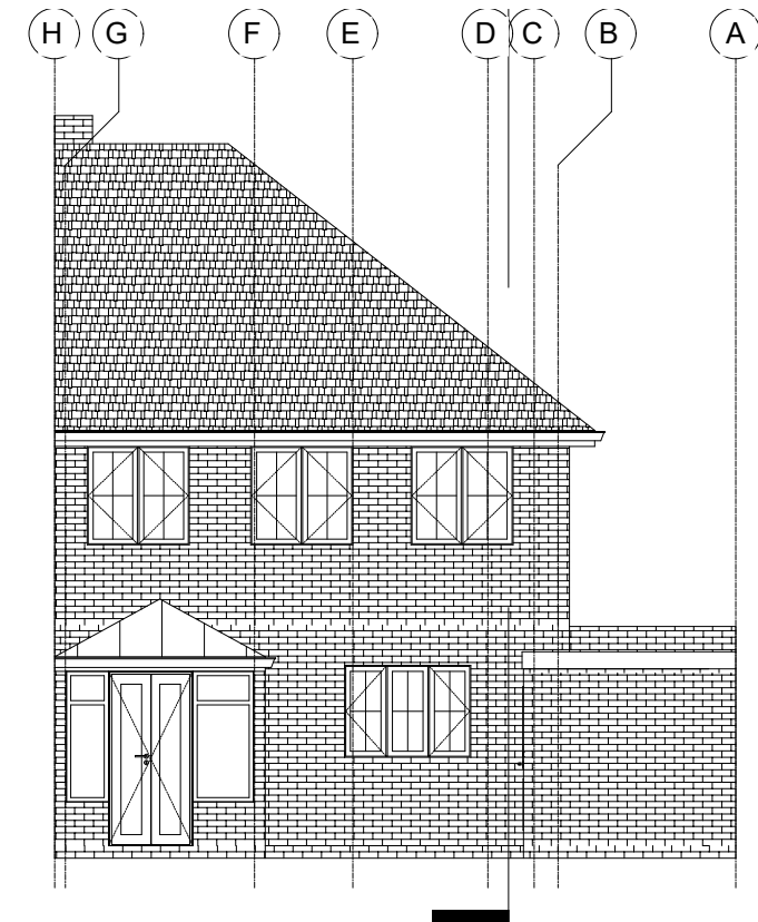
EXISTING REAR ELEVATION
