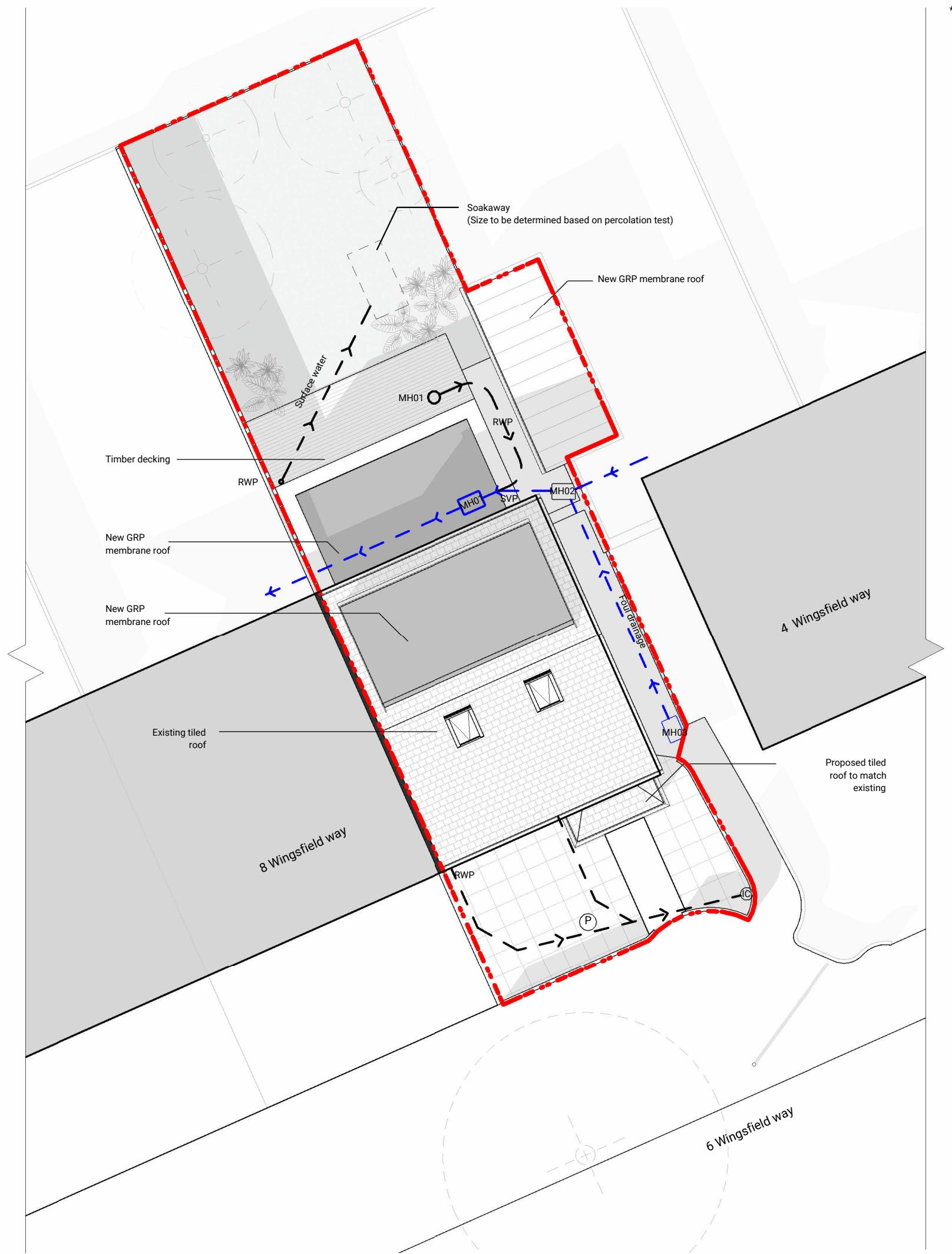
\*All new drainages should be connected to Proposed Manhole MH01
