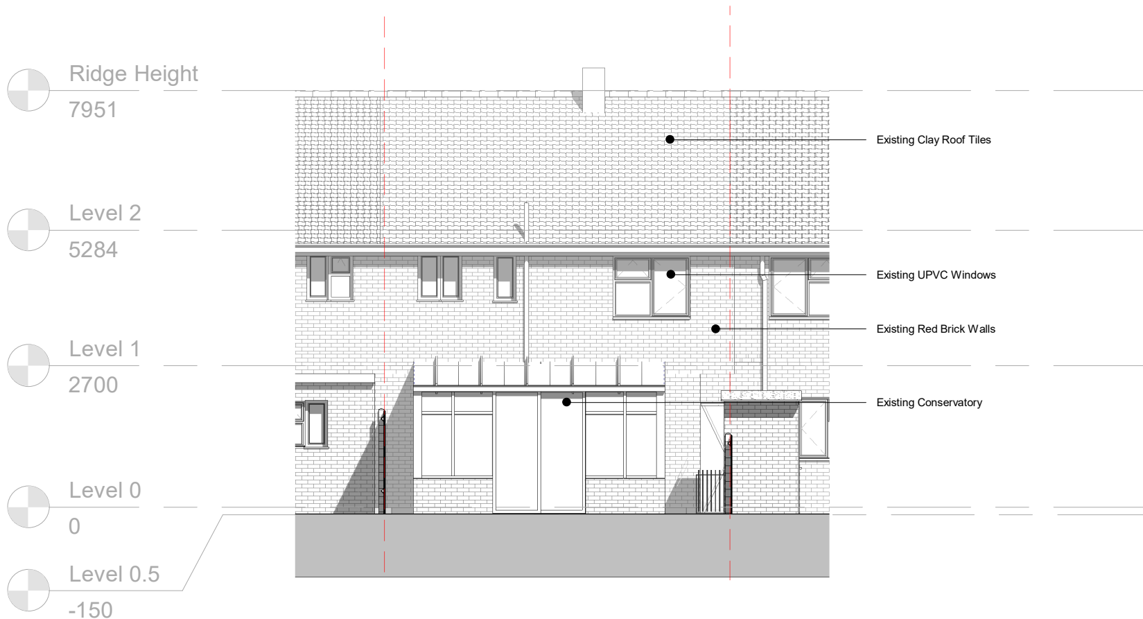
Existing Rear South Elevation 1 : 100
