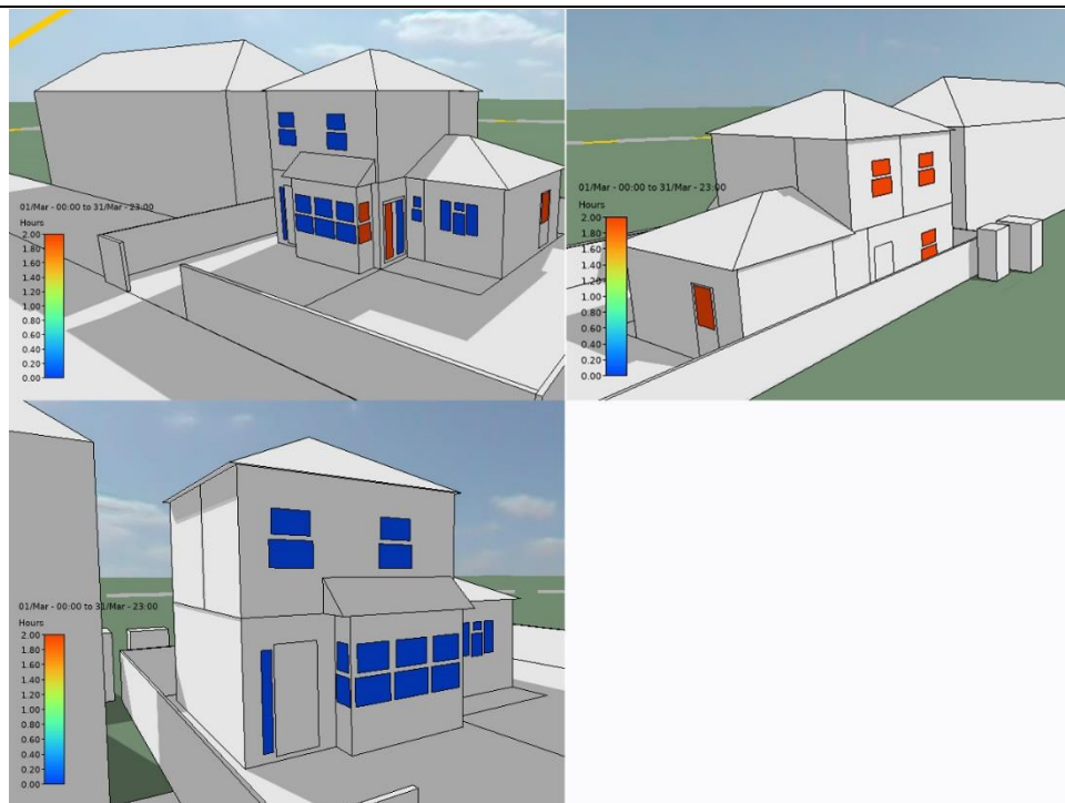
Figure 7. Direct Sunlight Hours analysis of window elements of the proposed development on 21st March as seen from (a) north view, (b) west view, and (c) rear view.
