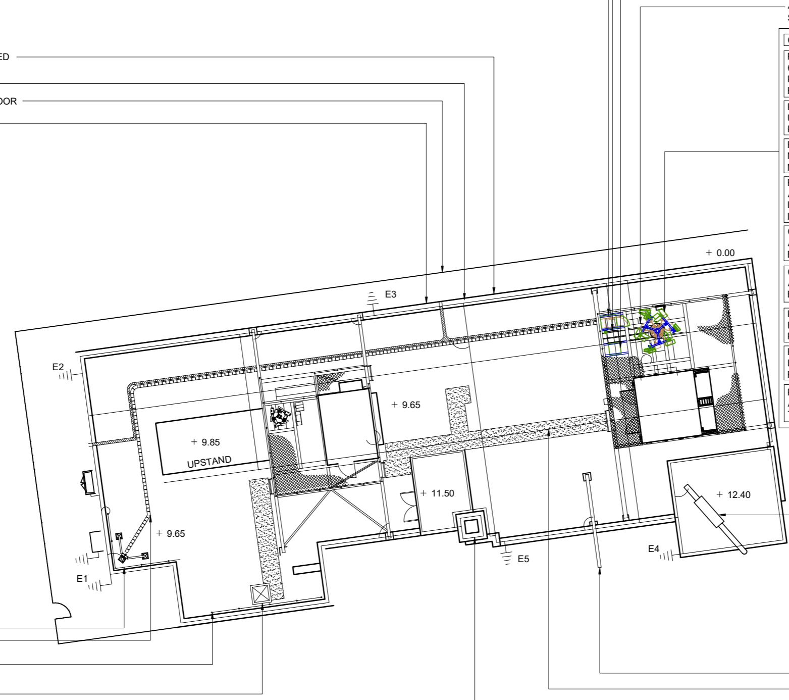
PROPOSED CTIL 1No. FLAT PACK FRAME TO BE INSTALLED ON GRILLAGE
