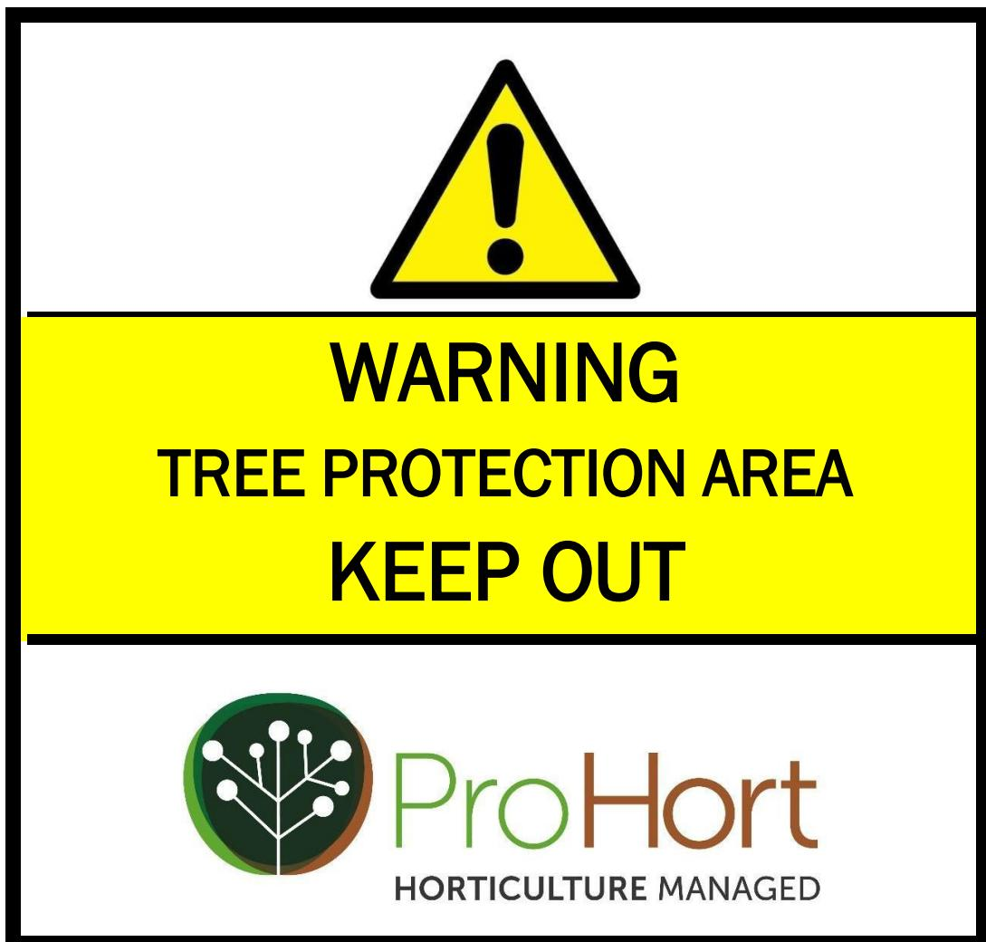
*This sign must be minimum A4 size and at 1.5 metres above ground level.*
