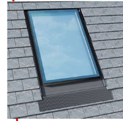
ROOF LIGHTS on pitch roof Rooflights to be double glazed + to meet 'U' value of min. 2.0 W/m sq.K. All roof lights to be A-A fire rated.
