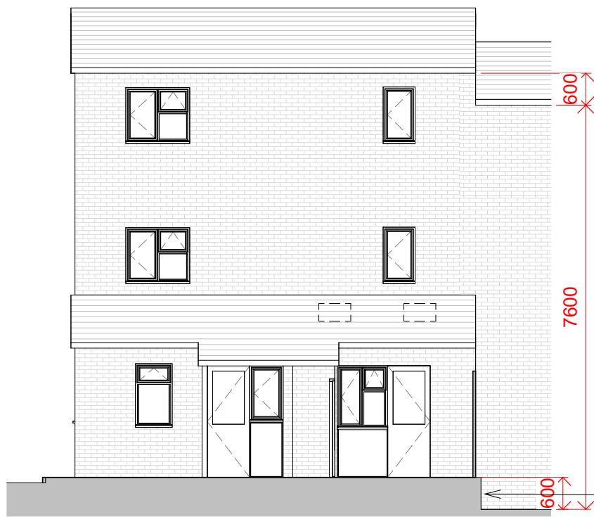
New storey added to have the same floor to ceiling height as existing storeys.
