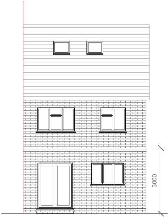
Proposed Rear Elevation Scale 1:100
