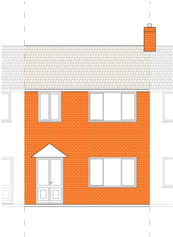
EXISTING FRONT ELEVATION scale 1:100
