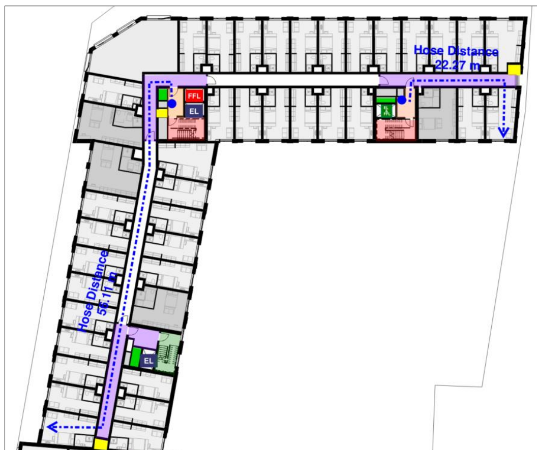
Figure 11: Hose Coverage – Typical Floor
