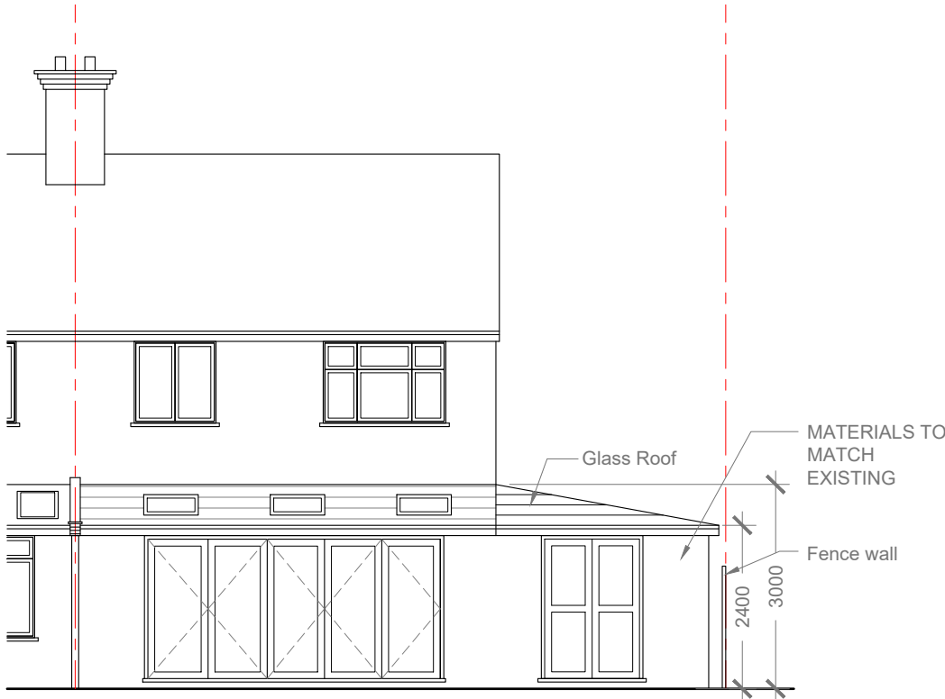
Proposed Rear Elevation Scale 1:100
