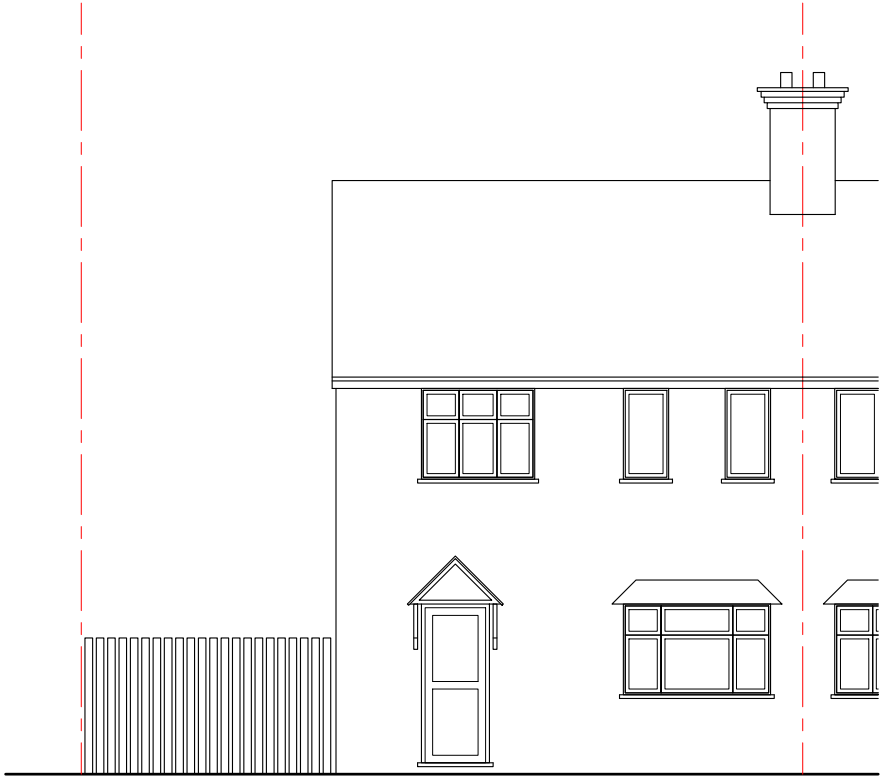
Existing Front Elevation Scale 1:100
