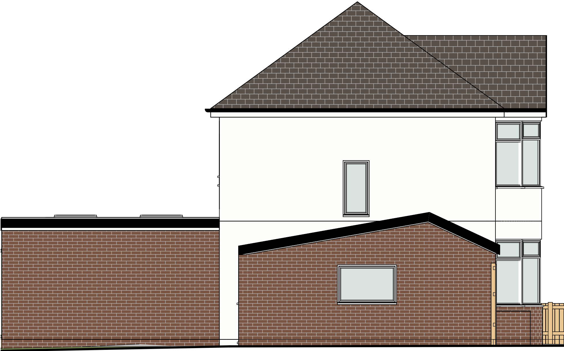
4 Proposed Left Side Elevation 1 : 50
