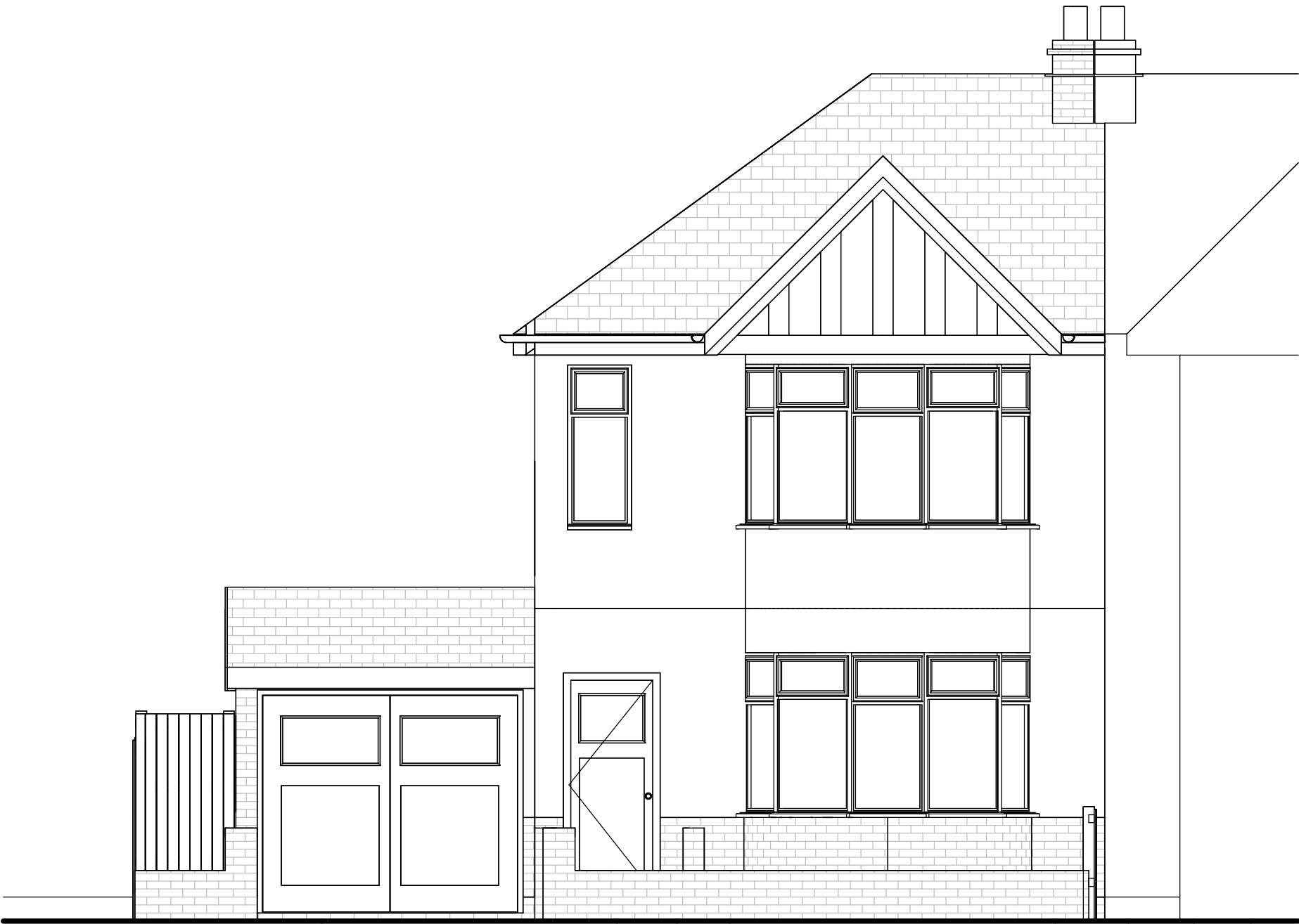
1 Existing Front Elevation 1 : 50
