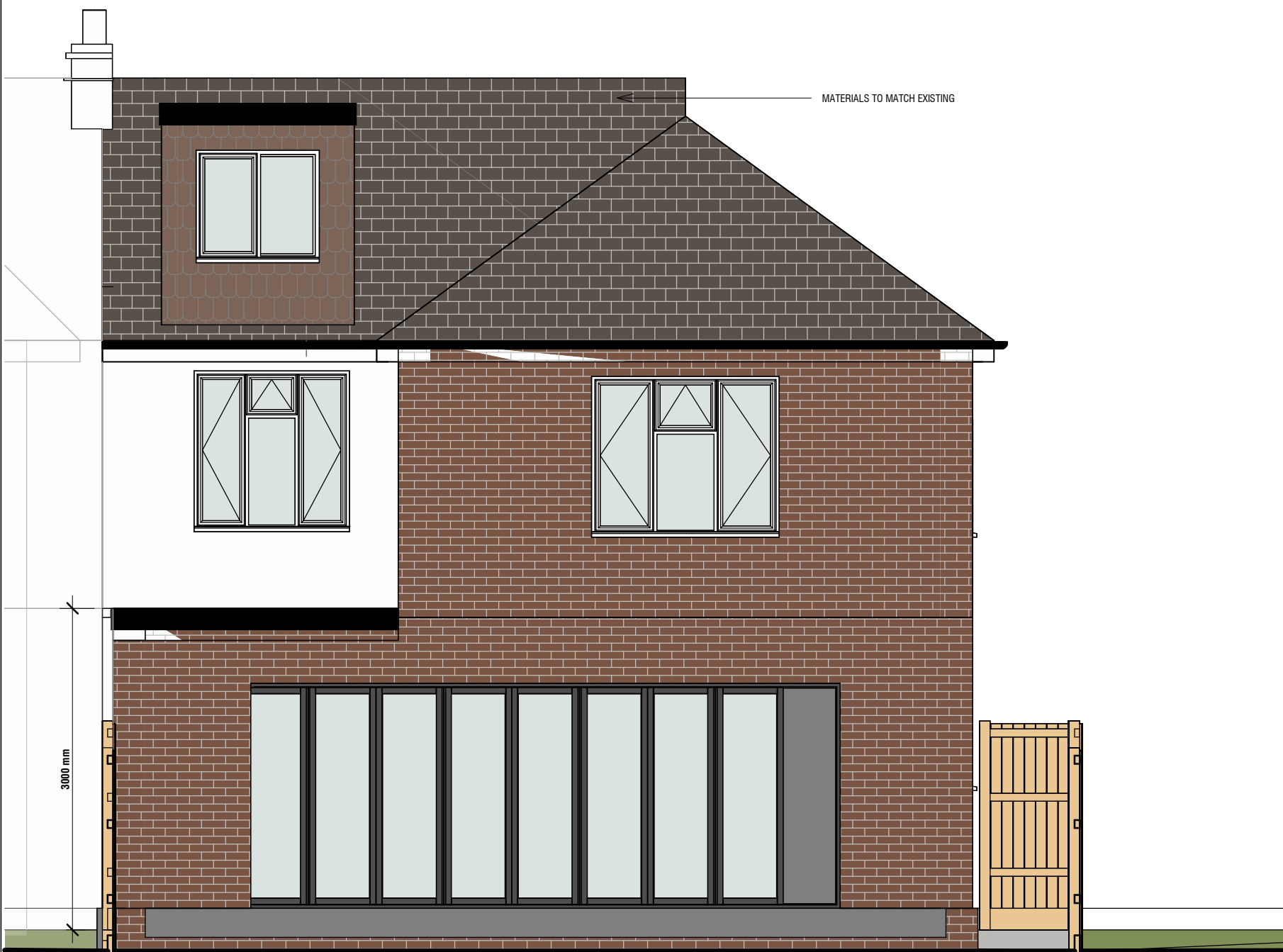
3 Proposed Rear Elevation 1 : 50
