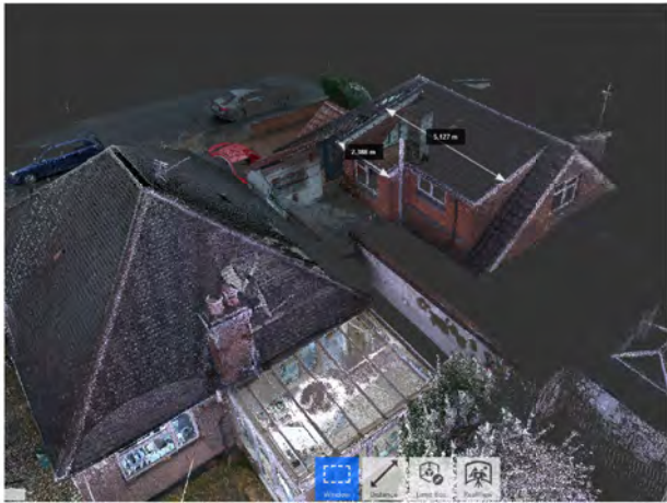
6. POINT CLOUD SURVEY OF DORMER AT NO.69 (with dimensions) survey completed on 08/02/24 using Leica BLK laser scanning hardware
